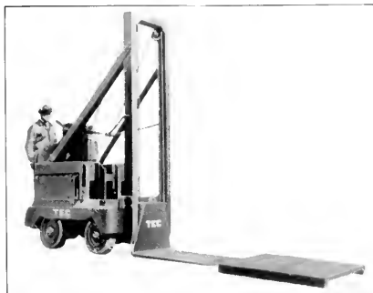
New TEC 4-wheel drive, storage battery truck for handling cargo on skids.
